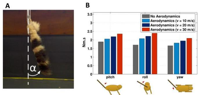
Fig. 2: (A) Cheetah fur placed in a wind tunnel. (B) Angular impulse for various motions with the aerodynamic effects included.
