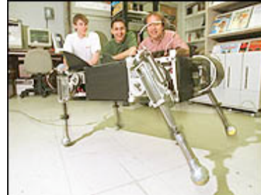
Scout II hops past student engineers Don Campbell and Martin de Lasa and mechanical engineering professor Martin Buehler
