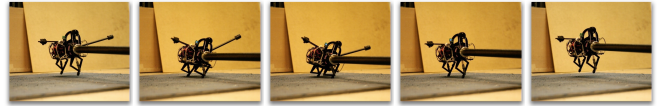
Fig. 1. Snapshots from apex to apex of tail-energized planar hopping (§V) implemented on a new robot platform—the Penn Jerboa (§VI).
