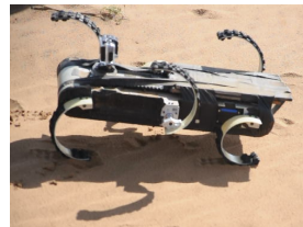
Figure 10: D-RHex with an 8.5kg steel plate for a payload.
