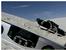
(b) The back left leg has stalled out and the robot is unable to make further progress at 27.05 degrees.
