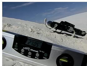
(c) The crawl pitched backwards far enough that the front two legs had difficulty making contact with the ground.
