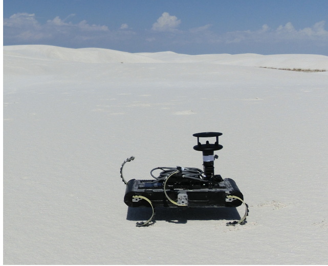
(b) The WindSonic mounted on D-RHex
