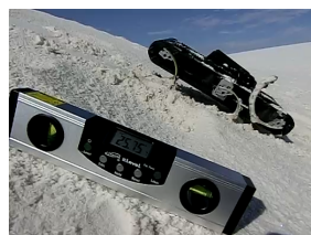
(a) A successful crawl ascent at 25.75 degrees of incline.
