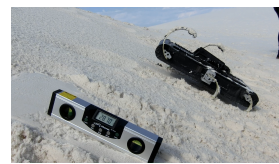
(f) The alternating tripod gait failed when rear leg motors stalled.
