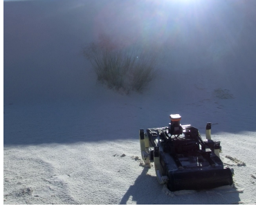
(a) D-RHex performing a pitching maneuver in front of a bush at White Sands.
