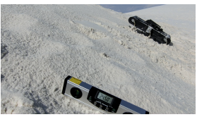
(e) Here the slow pronk is failing on softer, lighter sand at 24.50 degrees of incline.
