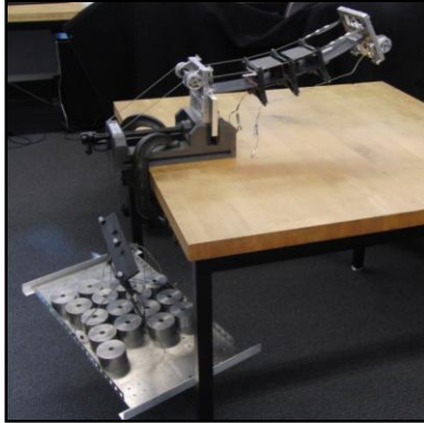
Figure 3: Weights were suspended from the spine cables imposing a gravitational load whose resulting flexion could be measured in the same units of cable lengths as accessible to actuators during physical operation. The change in potential energy of the system was calculated by multiplying the weight of the platform by its Vicon measured displacement giving the relationship between cable flexion displacement and potential energy stored.
