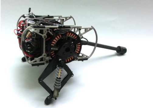
Figure 7. The Jerboa is a 2 Kg robot with hip-actuated legs and a 2DOF tail, pictured on the left as it appeared in the experiments of Section VI. On the right is our model for the planarized 4DOF system for comparison.
