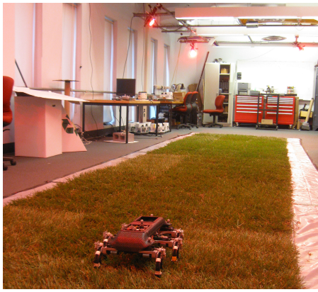
Fig. 8. Picture of EduBot on grass terrain.
