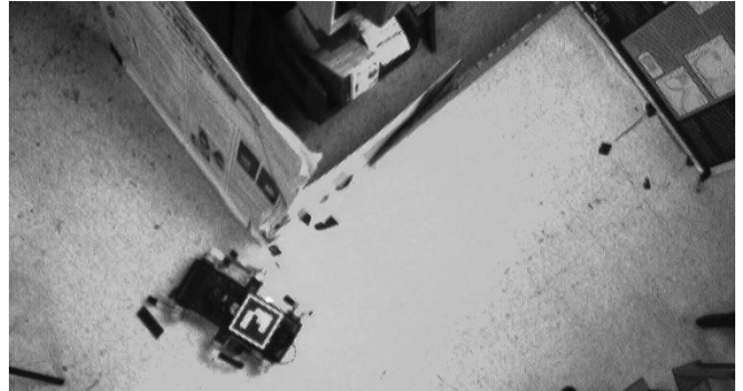
Fig. 1. Our experimental platform: a RHex variant (a hexapedal legged running platform whose horizontal plane dynamics is well approximated by the unicycle model (9) at modest speeds [16]) equipped with a conventional laser scanner idealized as an infinitesimal sensor, seen here tracking a wall as part of our test suite (cf. Section IV-A).
