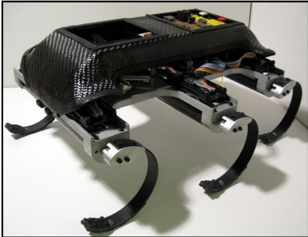
Figure 1. EDUBOT, A HEXAPEDAL DYNAMIC LEGGED LOCOMOTION PLATFORM [6].
