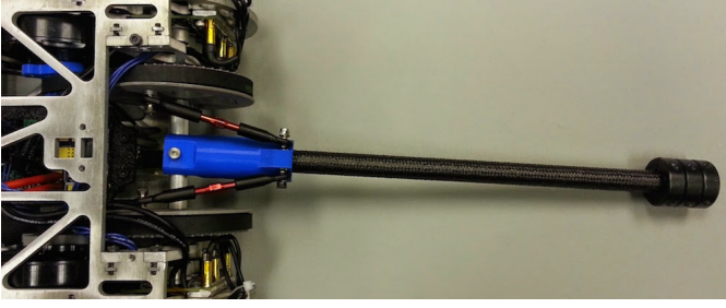
Figure 8: The jerboa tail is a 2DOF spherical joint controlled using coaxial motors through a mechanical linkage. Though there are driven sprockets visible in this image, the version of the robot presented in this paper did not have this additional reduction stage.
