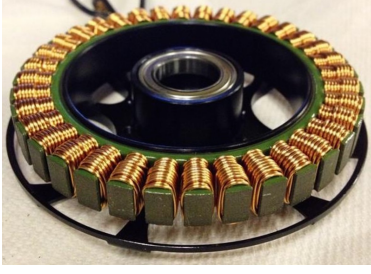
Figure 10: Left: The selected actuator for the Jerboa is the T-motor U8 , showing a thin profile and large gap radius—desireable properties for legged applications [35]. Middle: Motor properties relevant to selection for legged applications for the Jerboa motor, and the X-RHex [36] motor. Right: A torque-current plot for the U8 when coupled with our custom motor controllers of Fig. 11, showing flux saturation at higher currents and a dashed line for the nominal torque (predicted by K_T ).
