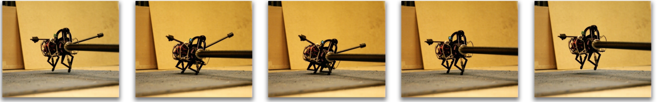
Figure 2: Snapshots from apex to apex of tail-energized planar hopping (§5) implemented on a new robot platform—the Penn Jerboa (§6).
