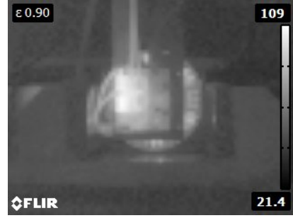
Figure 11: Left: The physical dimensions of our motor controller when compared to the motors they are driving. Right: Infrared image of our actuation setup at stall, showing the controller reaching higher temperatures than the motor coils.
