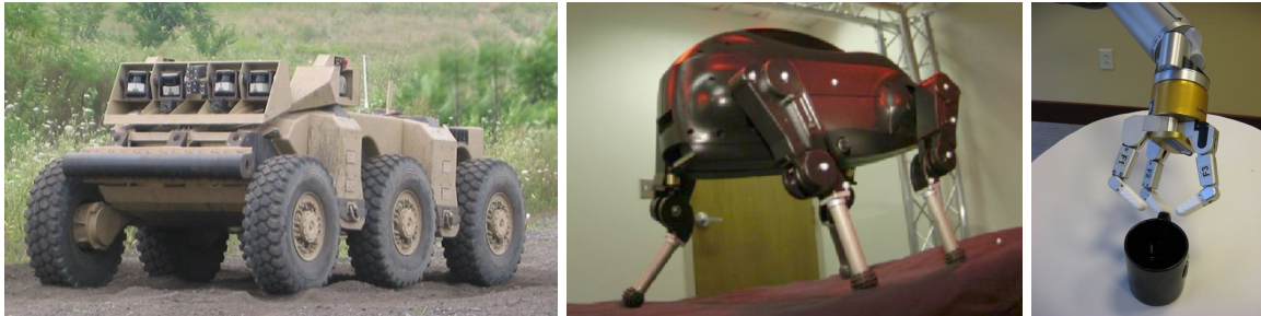
Figure 1: Imitation learning applies to a wide variety of robotic platforms. This figure shows a few of the robots on which the imitation learning algorithms discussed here have been implemented. From left to right, we have (1) an autonomous ground vehicle build by the National Robotics Engineering Center (NREC) known as Crusher, (2) Boston Dynamics’s LittleDog quadrupedal robot, and (3) Barrett Technologies’s WAM arm, wrist, and 10-DOF hand.
