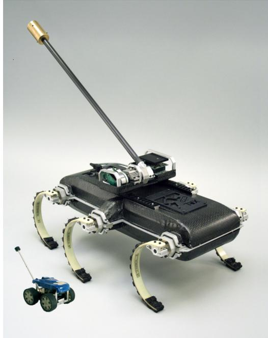
Figure 2.2: XRL [65] with a new tail, and with approximately sized image of Tailbot [32, 108]. *This figure originally appeared in [92] is included here courtesy of Tom Libby and Ryan Knopf.*
