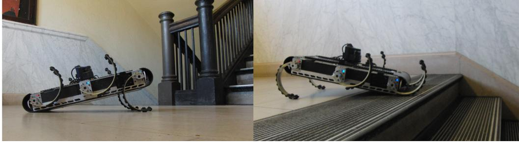
Figure 4.7: Robot performing two pitching sensor sweeps with a planar laser scanner: (Left) upward ( $\phi > 0$ ) to scan a staircase, (Right) downward ( $\phi < 0$ ) to check for a cliff.
